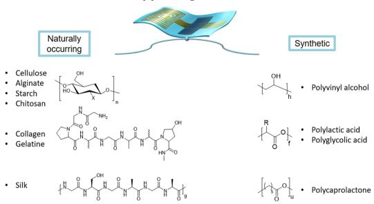
Fig. 4 Bioderived supporting materials for electronics-polysaccharides (cellulose, 48.56-58.65 alginate, 66-70 starch, 34.49 chitosan, 14.34,59-64), collagen, 71 silk 31.41-43.72 and synthetically derived supporting materials for electronics-polyvinyl alcohol (PVA), 14.16.17,73-75 polyglycolic acid (PGA), polylactic acid (PLA), 19-22.76 polycaprolactone (PCL), 26.27,38,77-79
