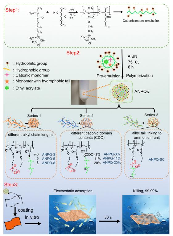
Scheme 1 Synthesis of ANPQs and antibacterial mechanism of ANPQ-treated fabrics.
