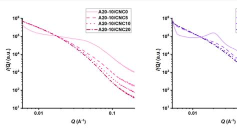
Fig. 4 1D-SAXS profiles of the PPU/CNC nanocomposites with varying PBLA and CNC content collected at room temperature for 30 minutes. The neat PPU matrices (i.e., A20-10/CNC0 and A20-20/CNC0) exhibit a defined scattering peak, whereas the addition of CNC to the matrices results in a reduction or loss of the distinct peak. These results indicate that the introduction of CNCs into PPU matrices modulates long-range ordering and structural hierarchy
