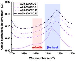
Fig. 2 ATR-FTIR spectra of PPU/CNC nanocomposites as a function of the CNC weight fraction. Peptide secondary structure was identified based on the second derivative in the amide I stretching region (1700-1600 cm<sup>-1</sup>). CNC incorporation into PPUs leads to variations in secondary conformation, disrupting \alpha-helical ordering but promoting intermolecular hydrogen bonding. This finding provides evidence of preferential interactions between the PBLA blocks and CNCs.
