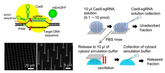
Fig. 10 Gene editing through the use of mechanically responsive mechanisms. The mophology of nanoneedle array and the schematic of RNP loading and releasing mechanism from the nanoneedles. Adapted from (Yamagishi et al. 2019). 144 © 2019 MDPI.
