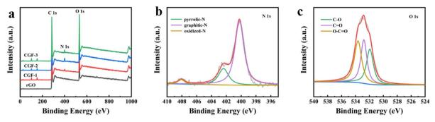
Fig. 6 (a) XPS spectra of rGO and composite film samples; (b) N 1s spectra of CGF-2; (c) O 1s spectra of CGF-2.
