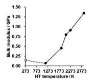
Fig. 8 The bulk modulus of CMS and its heat-treated samples. CMS is plotted at  $298~\mathrm{K}$  for a reference.
