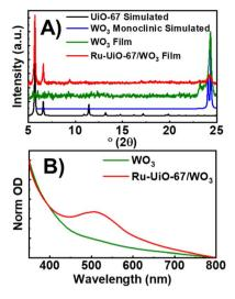
Fig. 1 (A) PXRD patterns of simulated UiO-67 (black), monoclinic WO<sub>3</sub> (red), WO<sub>3</sub> film (blue), and Ru-UiO-67/WO<sub>3</sub> (orange). (B) Ground-state absorption spectra of WO<sub>3</sub> (black), and Ru-UiO-67/WO<sub>3</sub> (red).
