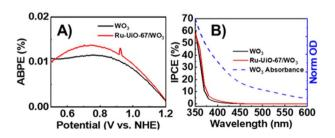
Fig. 3 (A) Photo-response efficiency of WO<sub>3</sub> (black) and Ru-UiO-67/ WO<sub>3</sub> (red) as a function of potential (ABPE). (B) Wavelength (IPCE) of WO<sub>3</sub> (black), Ru-UiO-67/WO<sub>3</sub> (red) measured under monochromatic light at 500 mV applied potential, overlaid  $WO_3$  absorption spectrum (blue dashed line).
