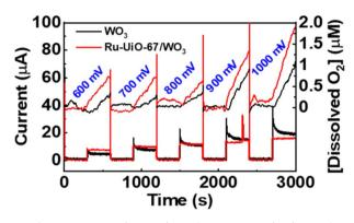
Fig. 8 Current increase (bottom) and  $O_2$  production (top) for  $WO_3$  and Ru-UiO-67/ $WO_3$  at different applied potentials. At each potential, the photoelectrode was held in the dark for 5 minutes before illumination for 5 minutes.
