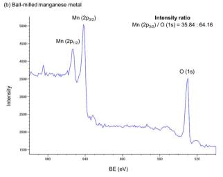
Fig. 2 X-Ray photoelectron spectra of commercial manganese metal (a) before ball milling and (b) after ball milling.
