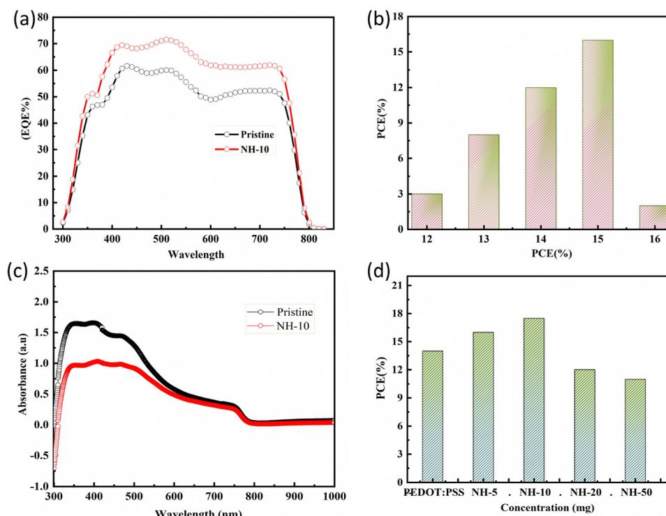
Fig. 2 Optoelectronic properties analysis (a) EQE spectra, (b) show the average value of PCE, and (c) UV-visible absorbance spectra for both pristine and  $\text{NH}_4\text{Cl}$ -10 doped PEDOT: PSS. (d) PEC of different doping concentrations.
