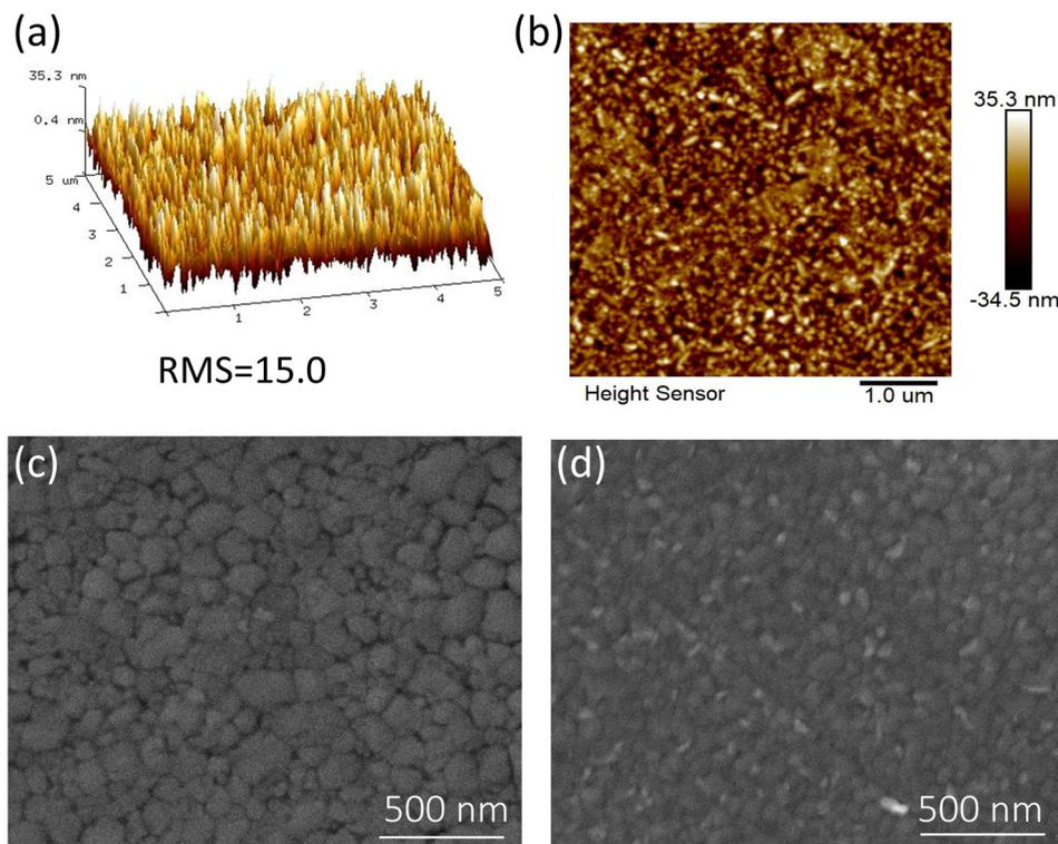
Fig. 3 Surface morphology analysis. (a and b) AFM topography of  $\text{NH}_4\text{Cl}$ -10 doped PEDOT: PSS, SEM images of perovskite films, (c) pristine, (d)  $\text{NH}_4\text{Cl}$ -10 PEDOT: PSS.
