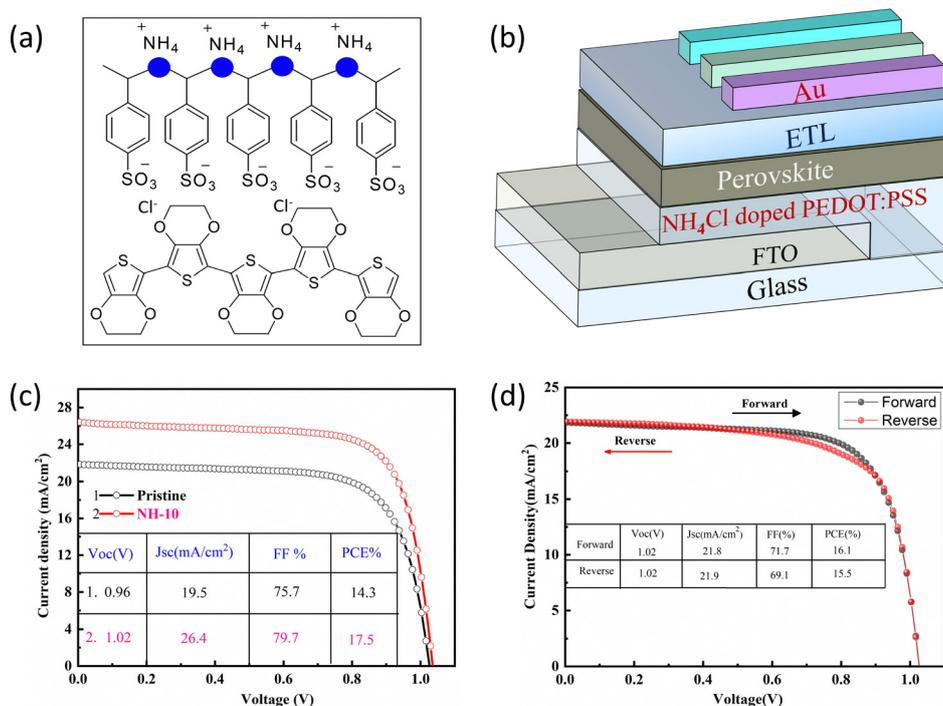
Fig. 1 (a) Chemical structure of PEDOT: PSS, (b) schematics diagram of PSCs, (c) typical  $J-V$  curves of the PSCs based on pristine and  $\text{NH}_4\text{Cl}$ -10 doped PEDOT: PSS, (d) reverse and Forward scan of the  $\text{NH}_4\text{Cl}$ -10 doped PEDOT: PSS-based PSCs.
