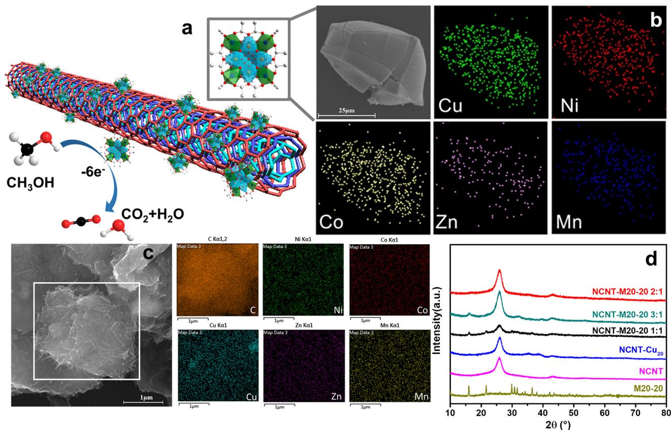
**Fig. 2** Structural characterizations of the NCNT-M20-20 composite. (a) Graphic illustration of NCNT-M20-20 2 : 1 in the MOR process, with the structure of M20-20 shown as a ball-stick model. (b) Morphology of M20-20 and mapping information of the selected area. (c) Morphology of NCNT-M20-20 2 : 1 and EDS results. (d) Powder XRD of a series of materials.
