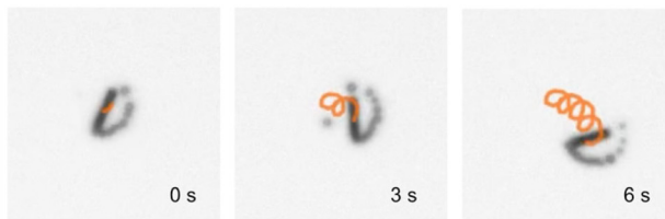
C Time lapse of MnO 2 /Lac micromotor trajectories at 2 wt. % H 2 O 2
