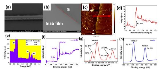
Fig. 3 (a) SEM image of the InSb-microfiber; (b) SEM graph of the InSb film on a Si substrate on 1 mm scale; (c) AFM graph; (d) the height profile; (e) the EDX spectra of InSb; (f) the full XPS spectrum of InSb; (g) the XPS spectrum of the Sb atom; and (h) the XPS spectrum of the In atom.
