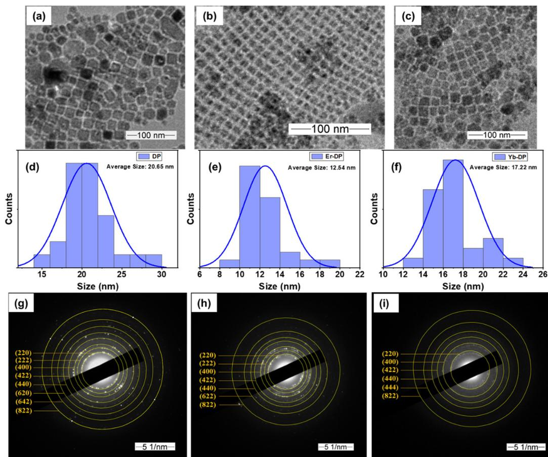
Fig. 2 Low magnification TEM images of (a) DP, (b) Er-DP and (c) Yb-DP. The average size of the corresponding NCs is shown in (d)–(f). SAED patterns of (g) DP, (h) Er-DP and (i) Yb-DP.
