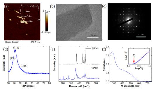
Fig. 1 Characterization of VP Ns. (a) AFM image of VP Ns and the height profile along the white line. (b) TEM image of VP Ns. (c) SAED image and (d) XRD pattern of VP Ns. (e) Raman spectra of VP and BP Ns. (f) UV-vis absorption spectrum of VP Ns in NMP solution; the inset is  $(\alpha_0 h \nu)^2$  versus photon energy  $h\nu$ .
