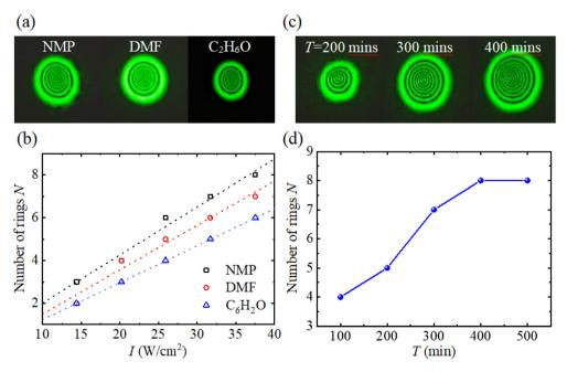
Fig. 2 (a) Complete ring patterns with VP Ns dispersed in three different solvents at  $I = 31.7 \text{ W cm}^{-2}$ . (b) Intensity dependence of the number of rings for VP Ns dispersed in three different solvents. (c) Complete ring patterns for VP Ns dispersed in NMP at I = 37.5 W cm<sup>-2</sup> with three ultrasonic times T. (d) T-Dependence of the number of rings for VP Ns dispersed in NMP at  $I = 37.5 \text{ W cm}^{-2}$ .
