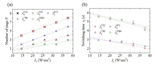
Fig. 7  $I_c$ -Dependent (a) ring number N and (b) switching time  $\tau_S$  for the signal beams at 532 nm, 671 nm, 780 nm, and 1064 nm with the control beam at 532 nm. The dotted lines are for visual guidance.
