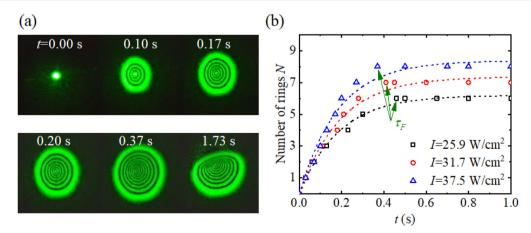
Fig. 3 (a) The self-diffraction ring patterns of VP nanosheet dispersion in NMP recorded at different times t with I = 37.5 W cm<sup>-2</sup>. (b) The evolution of the number of rings N over time t at three different intensities.
