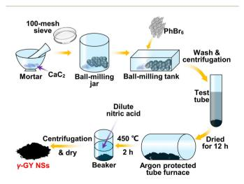
Fig. 1 Preparation flow chart of  $\gamma$ -GY NSs.
