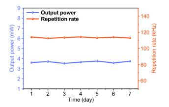
Fig. 7 Variation of the output power and repetition rate of the QSFLs
