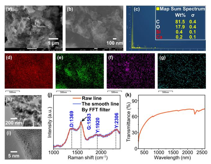
Fig. 2 (a) SEM image at a scale of 1 μm. (b) SEM image at a scale of 100 nm. (c) Atomic ratio of  $\gamma$ -GY NSs. EDS images of  $\gamma$ -GY NSs corresponding to (d) C, (e) O, (f) Si and (g) Ca, respectively. (h) TEM image and (i) HRTEM image of  $\gamma$ -GY NSs. (j) Raman spectrum of  $\gamma$ -GY NSs. (k) VIS-IR transmission spectrum of  $\gamma$ -GY NSs.
