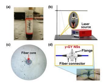
Fig. 3 (a) A photograph of a  $\gamma$ -GY NS dispersion. (b) Experimental setup of the laser-induced deposition method. (c) Micrograph of a fiber facet with  $\gamma$ -GY NSs after optical deposition. (d) Self-assembly conducted for a  $\gamma$ -GY-SA. Inset: the schematic of the  $\gamma$ -GY-SA.
