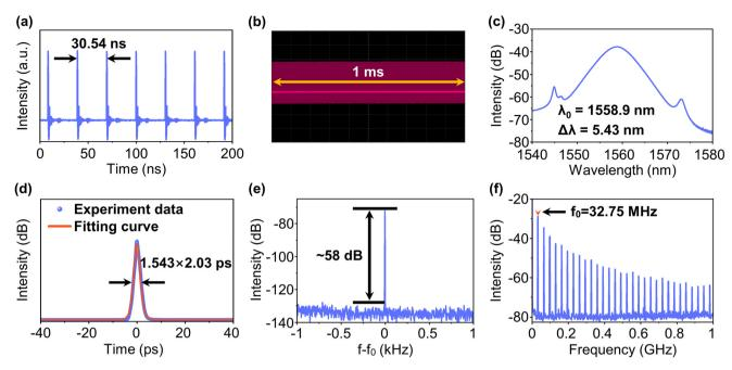
Fig. 8 (a) Temporal pulse trains and (b) oscilloscope trace within 1 ms. (c) The optical spectrum. (d) Autocorrelation trace with sech<sup>2</sup> pulse profile. (e) RF spectrum over a 2 kHz span with a resolution bandwidth of 1 Hz at the fundamental frequency and (f) the wideband RF spectrum with 100 kHz resolution.  $\Delta\lambda$ : 3 dB bandwidth;  $f_0$ : fundamental frequency.
