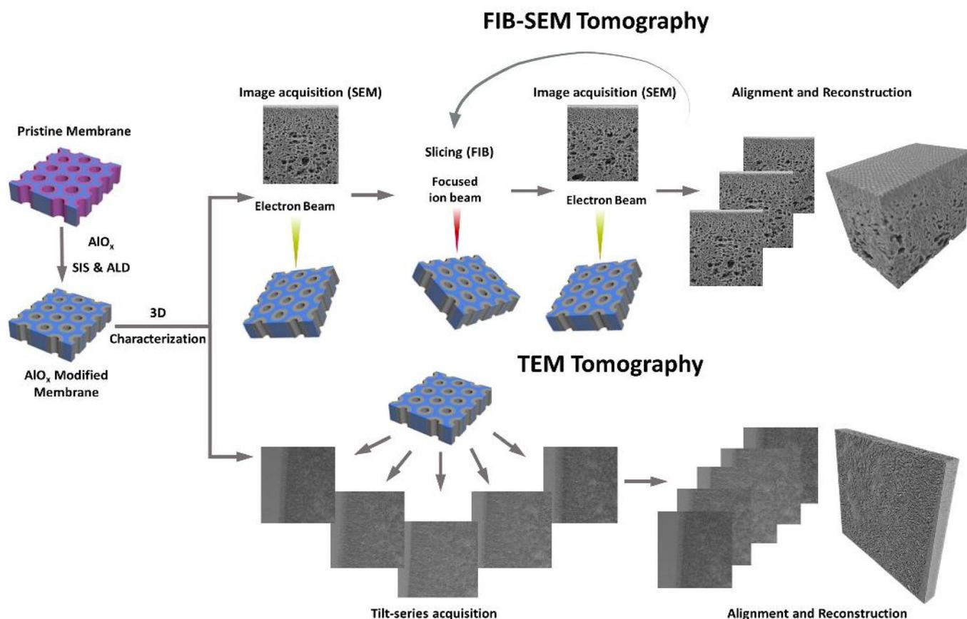
**Fig. 2** Illustration of the 3D characterization process:  $\text{AlO}_x$  is selectively grown in the P4VP pore-forming domain by SIS, followed by additional cycles of  $\text{AlO}_x$  ALD. This enhances the contrast, allowing for both FIB-SEM tomography and TEM tomography with high detail and resolution.
