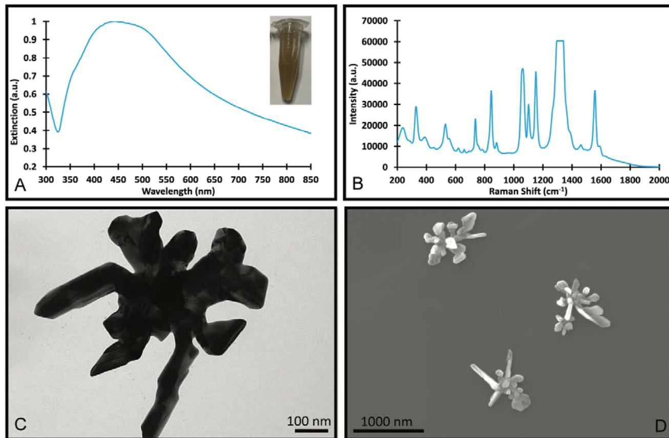
Fig. 5 UV-Visible spectrum (A), SERS spectrum (B), TEM Image (C) and SEM images (D) of the SERS nanosupernova formed with 90  $\mu\text{L}$  of 10 mM  $\text{AgNO}_3$  and 30  $\mu\text{L}$  of hydroquinone and incubated for 12 h.
