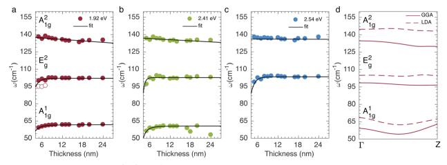
Fig. 2 (a-c) The frequency position of  $A_{1q}^2$ ,  $E_q^2$ , and  $A_{1q}^1$  modes as a function of QL thickness for excitation laser energies of 1.92, 2.41 and 2.54 eV, respectively. The lines in  $A_{1q}^1$  and  $E_q^2$  modes are a guide to the eye. (d) DFPT calculation of phonons dispersion a long of  $\Gamma - Z$  direction employing the LDA and GGA approximations.
