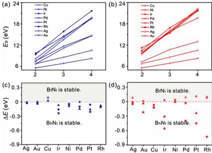
Fig. 3 Binding energies as a function of BN clusters terminated with (a) N and (b) B atoms. The difference in formation energy between  $B_h N_t$  and B<sub>f</sub>N<sub>t</sub> of (c) N and (d) B terminated BN clusters. Squares, stars, and triangles represent the cluster size of 2, 3, and 4, respectively. 180
