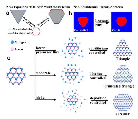
Fig. 6 (a) Kinetic Wulff model of h-BN evolution, exhibiting the preferred progression from triangle to truncated triangle with increasing boron chemical potential. (b) Nonequilibrium dynamics of h-BN development calculated from a phase field simulation, representing the triangle and circular shapes under low and high precursor flux, respectively. (c) Schematic representation of the progression of the h-BN pattern.<sup>257</sup>
