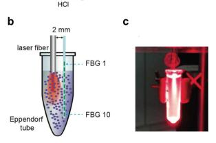
Fig. 1 (a) Schematic illustration of the synthetic route used to produce Au NRs; (b) experimental setup used to perform NIR irradiation of the Au NR samples and to measure the attained temperature distribution in real time; (c) picture of the sample under NIR irradiation. The visible red light is emitted from a pilot source.
