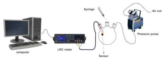
Fig. 1 Gas sensing setup.
