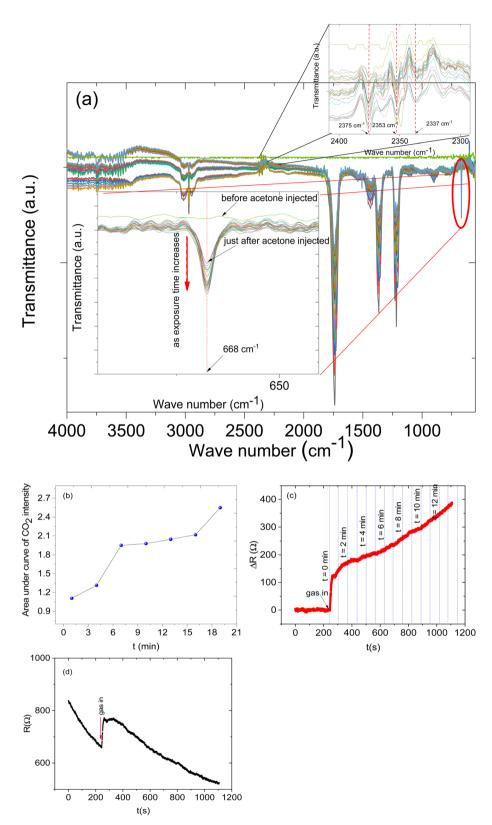
Fig. 10 (a) In situ FTIR: (b) areas under the curve of the CO<sub>2</sub> IR intensities against time (selected) (min), (c) the relative response of the sensor during the in situ FTIR coupled with LCR meter measurement and (d) transient response of the sensor during the in situ FTIR coupled with LCR meter measurement.
