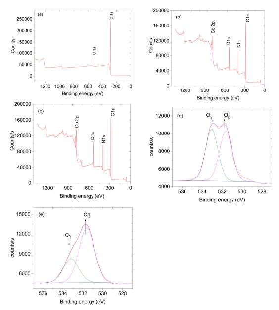
iig. 5 XPS spectra and XPs survey of (a) CNTs, (b) ZIF-67 and (c) ZIF-67/CNPs and (d) O 1s of CNPs and (e) O 1s of ZIF-67.
