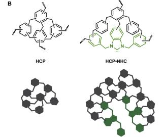
Fig. 1 (A) left to right: general structure benzimidazole based NHC, NHC@AuNP on solid support and AuNP supported in NHC containing support structure. (B) Structure and schematic of HCP/HCP·NHC structures.
