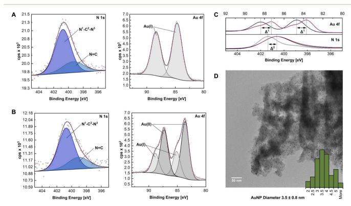
Fig. 2 (A and B) High resolution N 1s and Au 4f scans of HCP·NHC–Au(i) and HCP·NHC@AuNP respectively; (C) comparison of N 1s and Au 4f scan and corresponding  $\Delta^{1/2}$  via envelopes of HCP·BIMZ (gray), HCP·NHC–Au(i) (black) and HCP·NHC@AuNP (red); (D) TEM micrograph of HCP·NHC@AuNP.
