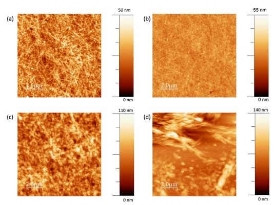
Fig. 6 AFM topography images of thin films deposited onto glass substrates using (a) BEDOTPy/NOSbF<sub>6</sub>, drop-cast,  $R_a = 6.7$  nm (b) BEDOTPy-EtOH-I/ NOSbF<sub>6</sub>, drop-cast R<sub>a</sub> = 3.0 nm, (c) BEDOTPy-EtOH-I/NOPF<sub>6</sub>, drop-cast, R<sub>a</sub> = 14.2 nm and (d) BEDOTPy-EtOH-I/NOPF<sub>6</sub>, spin-coated, R<sub>a</sub> = 17.3 nm.
