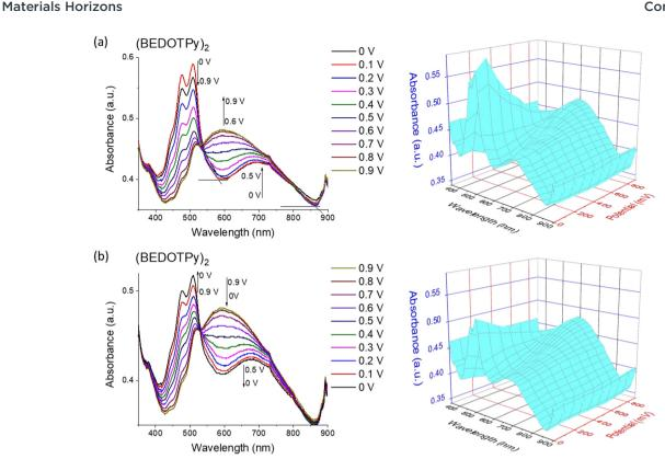
Fig. 4 Spectroelectrochemistry plots for (BEDOTPy)<sub>2</sub> in solid state show: (a) increasing the potential from 0 to +0.9 V and (b) decreasing it back to 0 V, using 3:1 v/v of acetonitrile and DCM dry solvents at scan rate 0.1 V s<sup>-1</sup>. Note: The spectra are not referenced to the Fc/Fc<sup>+</sup> couple.
