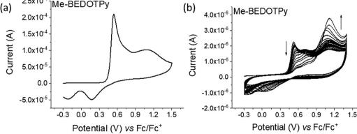
Fig. 2 Cyclic voltammograms referenced to the ferrocene redox couple for: (a) oxidation of Me-BEDOTPy, and (b) repetitive cycling (40 scans) over the oxidation range of Me-BEDOTPy. Conditions: Pt disk as working electrodes, Pt wire as a counter electrode and Ag wire as a reference electrode in ca. 0.1 mM of the compound in DCM with TBAPF<sub>6</sub> (0.1 M) as electrolyte at a scan rate of 0.1 V s $^{-1}$ .
