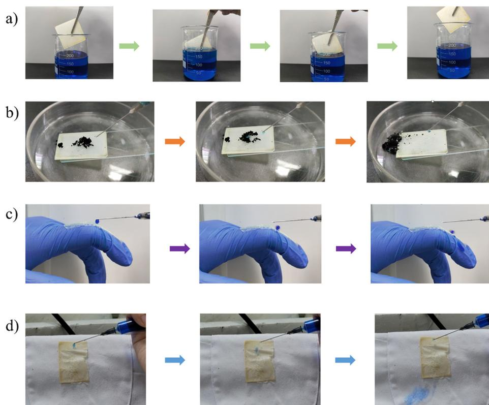
Fig. 12 The immersed and lifted-out behaviors of the PAI-TPU/m-SiO<sub>2</sub> surface in a blue dye solution of water (a). Self-cleaning test of the scuffed PAI-TPU/m-SiO<sub>2</sub> superhydrophobic surface (b). The wetting behavior of the stretchable PAI-TPU/m-SiO<sub>2</sub> superhydrophobic surface attached to an index finger (c) and lab coat (d).
