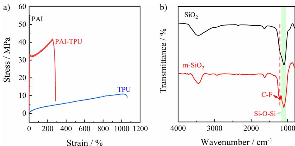
Fig. 1 Mechanical curves of PAI (black line), PAI-TPU stretchable substrate (red line) and TPU (blue line) films (a). FTIR curves of SiO<sub>2</sub> (black line) and m-SiO<sub>2</sub> (red line).
