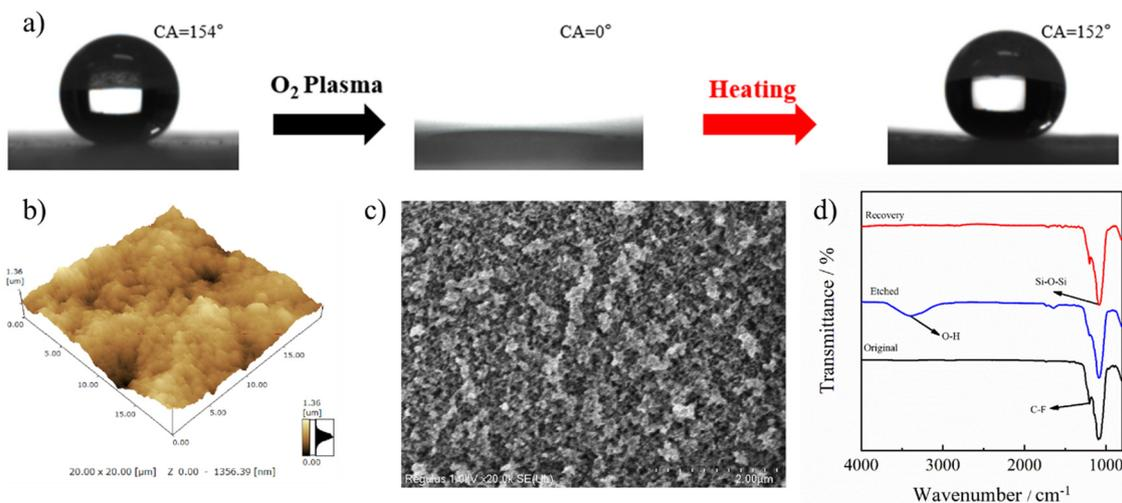
Fig. 10 The effect of O<sub>2</sub> plasma etching and heating treatments on the wetting behavior of the stretchable PAI-TPU/m-SiO<sub>2</sub> superhydrophobic surface (a). AFM 3D (b) and SEM (c) pictures after O<sub>2</sub> plasma etching treatment. The FTIR spectra of the PAI-TPU/m-SiO<sub>2</sub> superhydrophobic surface before (black line) and after (blue line) O<sub>2</sub> plasma etching treatment, and after heating treatment (red line) (d).
