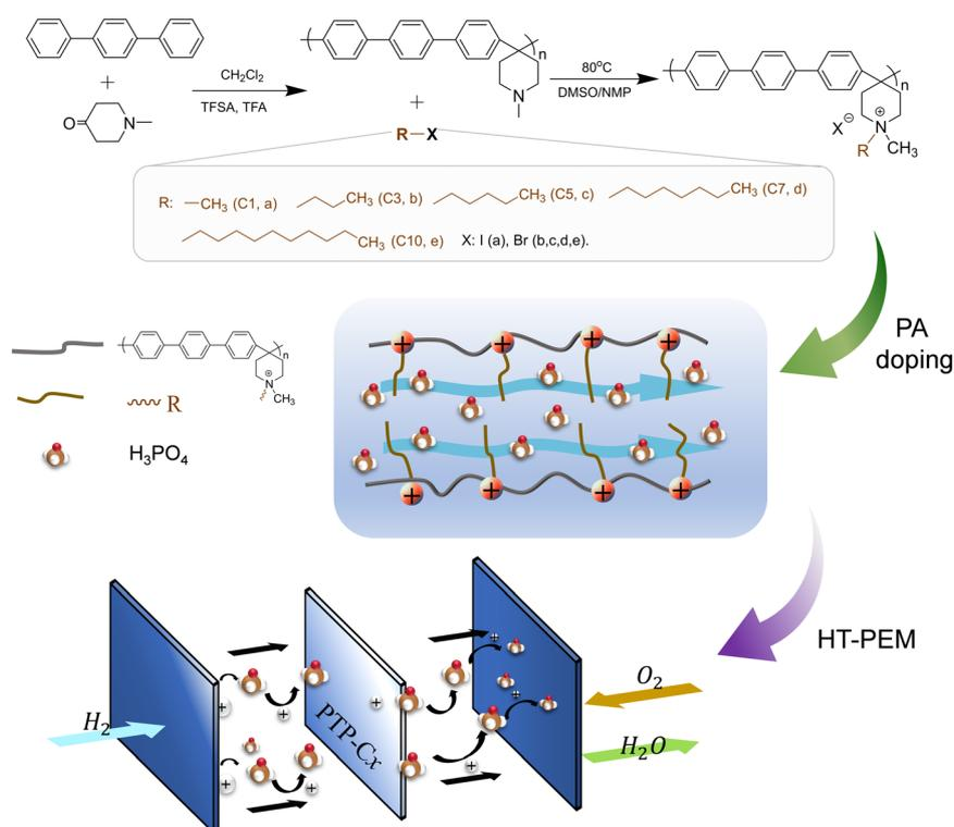
Fig. 7 Synthesis of PTP and fabrication of PTP-C<sub>x</sub> membranes.
