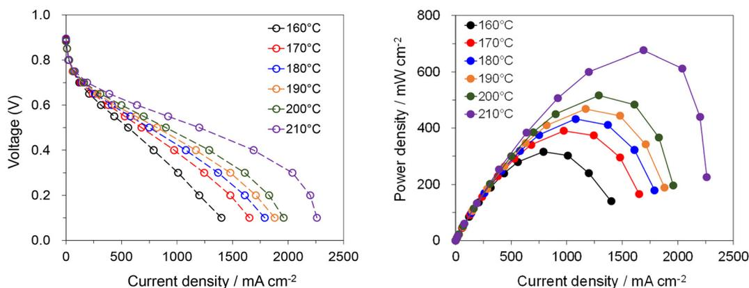
Fig. 6 Unhumidified H<sub>2</sub>-air fuel cell performances of the cell assembled with the PTP-C5/202% PA membrane without backpressure at different temperatures. The Pt catalyst loading in both electrodes was 1.5 mg cm<sup>-2</sup>.
