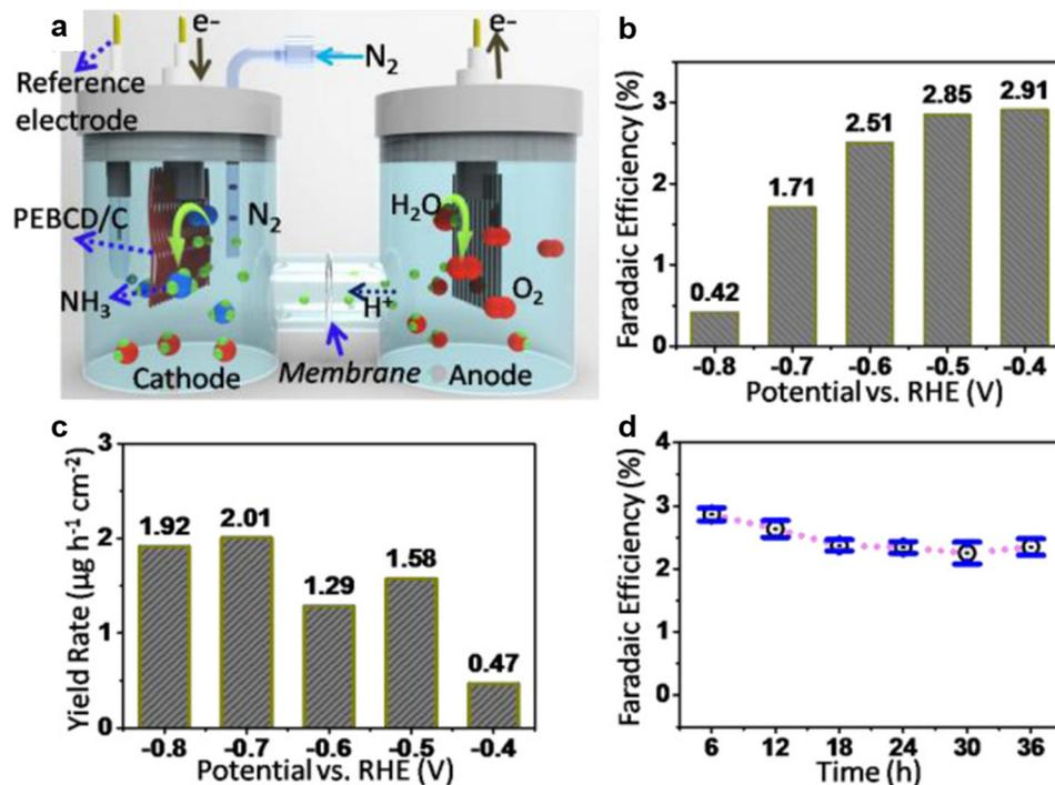
Fig. 11 (a) The graphic illustration of the configuration of the electrochemical cell for the  $eN_2RR$  process; (b) FEs of the  $Li^+$ -PEBCD/CC catalyst at different potentials during the  $eN_2RR$ ; (c)  $NH_3$  yield rate against applied potential during the  $eN_2RR$ ; (d) durability test results for  $Li^+$ -PEBCD/CC.<sup>3</sup>
