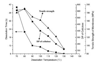
Fig. 8 Effect of dissolution time and temperature on the tensile strength and degree of polymerisation (DP) of regenerated cellulose (dissolved in [Bmim][Cl], regenerated in water). Reproduced from ref. 95 with permission from Wiley, copyright 2012.
