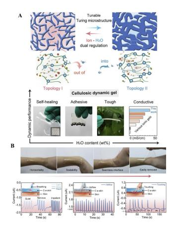
Fig. 23 (A) Transition between two topological networks by adjusting the water content of a cellulose/[Bmim][Cl] ionogel. The ionogel thus exhibits tunable dynamic properties as shown in the bottom of the figure. (B) Application of the dynamic ionogel in an electronic skin device that can be used for sensing e.g., breathing pattern, airflow and touching. Reproduced from ref. 205 with permission from Elsevier, copyright 2019.
