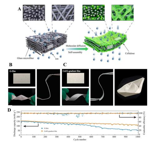
Fig. 15 (A) Fabrication of cellulose/glass microfiber composite film for application as separator in lithium-batteries. (B) Glass microfiber film with poor flexibility. (C) Cellulose/glass microfiber composite film with excellent flexibility and formability. (D) Cycling stability of a LiFePO<sub>4</sub>/Li cell using glass microfiber (blue line) vs. cellulose/glass microfiber composite (orange line) separators. Reproduced from ref. 149, copyright 2021 The Authors.
