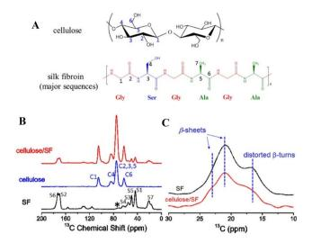
Fig. 19 (A) Structure of cellulose and silk fibroin with numbering for peak assignment (below). (B) <sup>13</sup>C CP/MAS NMR spectra of regenerated silk fibroin (SF), cellulose and cellulose/silk fibroin composite (3/1). Asterix indicates spinning sideband. (C) <sup>13</sup>C NMR spectra of regenerated SF and cellulose/SF composite in the Ala  $^{13}$ C $_{\beta}$  region for comparison. Reproduced from ref. 180 with permission from the American Chemical Society, copyright 2017.
