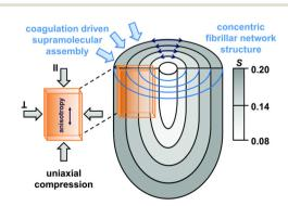
Fig. 28 Cellulose gel with concentric onion-like layers that have different level of ordering as shown with the *S* parameter, which indicates higher degree of ordering from the core towards the skin layer. Reproduced from ref. 236 with permission from The Royal Society of Chemistry, copyright 2019.
