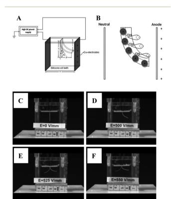
Fig. 21 (A) Experimental setup for studying the bending response of the ionogel under an applied electric field. (B) Schematic representation of the proposed mechanisms of the bending response. (C and D) Deflection and (E and F) swinging movement of the ionogel in response to a ground and positive electric field at room temperature. Reproduced from ref. 201 with permission from Elsevier, copyright 2012.
