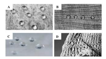
Fig. 31 Hydrophobic loncel-F fibres with 10 wt% (A and B) betulin and betulinic acid (C and D). Left pictures are nonwovens, right pictures are hand loomed/knitted fabrics. Reproduced from ref. 294, copyright 2021 The Authors.
