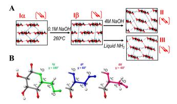
Fig. 2 (A) Formation of polymorphs under certain conditions. Arrows indicate the chain polarity, which is antiparallel for cellulose II. Chain orientation is shown on the a-b plane of the unit cell. (B) Possible conformations of the hydroxymethyl groups ( $-CH_2-OH$ ), tg: trans-gauche, gt: gauche-trans, gg: gauche-gauche.  $\chi$  indicates angles between the C5-O5 and C6-O6 bonds. Reproduced from ref. 10 with permission from Springer Nature, copyright 2019.
