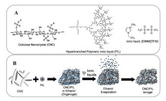
Fig. 24 (A) lonogel containing cellulose nanocrystals, hyperbranched polymeric ionic liquid and [Emim][NTf2]. (B) Method to prepared the CNC/PIL ionogel containing [Emim][NTf2]. Note that TFSI = NTf2. Reproduced from ref. 211 with permission from Wiley, copyright 2021.
