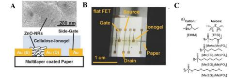
Fig. 22 (A) The structure of the ionic liquids used to fabricate the ionogels for electrolyte-gated field-effect transistor (FET) devices. (B) Schematic description of the flexible FET device with ZnO nanorods (NRs; an SEM image is shown above the device) and cellulose ionogel. (C) Photograph of the flexible paper-based FET. Reproduced from ref. 202 with permission from Wiley, copyright 2013.
