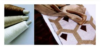
Fig. 30 (Left) loncell-F fibres produced using bleached pulp (white), cardboard (beige) and pulp with lignin as colorant additive (brown). (Right) Fabrics produced from the upcycled Ioncell-F fibres. Reproduced from ref. 264 with permission, copyright 2016 The Authors. Design: Marjaana Tanttu; photos: Eeva Suorlahti.
