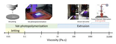
Fig. 2 Rheological considerations of polymer additive manufacturing processes. (PBF is not included here as viscosity alone is not the right framework for assessing a sintering process).
