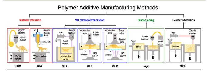
Fig. 1 Description of polymer additive manufacturing methods. Reproduced from ref. 32 with permission from American Chemical Society, 2021.
