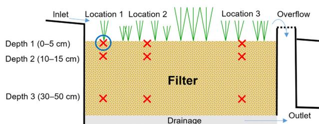
**Fig. 1** Schematic sketch of the sampling strategy in bioretention filter media with sampling points at three locations and at three depths, as marked by a red "X." The sequential extraction and pH analysis were performed at location 1 at depth 1, as marked by a blue circle.
