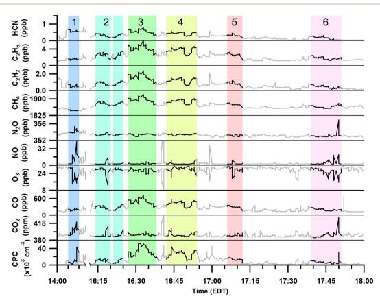
Fig. 2 Time series of 20 s averaged HCN,  $C_2H_6$ ,  $C_2H_2$ ,  $CH_4$ ,  $N_2O$ , NO,  $O_3$ , CO, and  $CO_2$  mole ratios and total particle (CPC) number concentrations over the full prescribed burn sampling period. Identified periods of smoke plume sampling are highlighted and numbered. Areas that are greyed out were not included in the plume analyses (Table 2).
