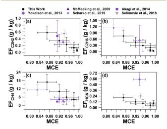
Fig. 3 Average emission factors for (a)  $C_2H_2$ , (b)  $C_2H_6$ , (c)  $CH_4$ , and (d) HCN versus MCE values for the six smoke plume periods, as well as previous studies. Error bars represent the 95% confidence interval for each calculated value. Previous values are from McMeeking et al.,6 Akagi et al., 15 Yokelson et al., 17 Scharko et al., 18 and Selimovic et al. 26
