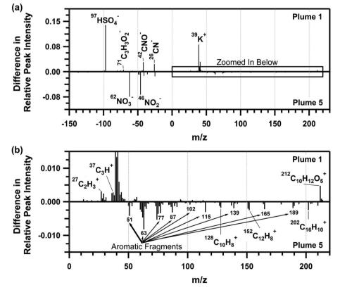
Fig. 6 (a) ATOFMS positive and negative ion mass average spectrum and (b) expanded positive ion mass spectrum for biomass burning particles during plume 5 subtracted from biomass burning particles during plume 1. Positive relative peak intensities correspond to greater abundance during plume 1; negative relative peak intensities correspond to greater abundance during plume 5. Only ion peaks above 95% confidence limits following subtraction are shown.
