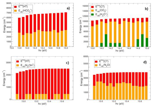
Fig. 6 Energy content of the products formed in the reaction involving CO<sub>2</sub><sup>+</sup> + H<sub>2</sub>O in HT (a) and CT channels (b). Energy content of the products formed in the reaction involving N<sub>2</sub>O<sup>+</sup> + H<sub>2</sub>O in HT (c) and CT channels (d)
