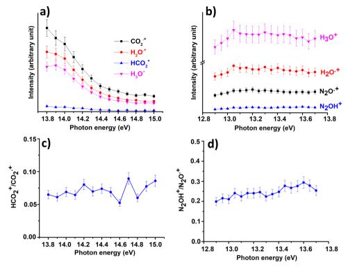
Fig. 3 Intensities of the ions involved in the reactions of Scheme 1 with  $X = CO_2$  (a) and  $X = N_2O$  (b) and the ratio  $HCO_2^+/CO_2^{\bullet+}$  (c) and  $N_2OH^+/N_2O^{\bullet+}$ (d) as a function of photon energy at the water pressure of  $4.3 \times 10^{-5}$  mbar and  $8.2 \times 10^{-5}$  mbar, respectively and CE = 0. Error bars are 10% of the values.
