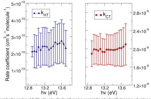
Fig. 5 Rate coefficient for the reaction of  $N_2O^+$  with water. On the left panel is reported the k for the HT channel as a function of the photon energy. On the right panel the rate coefficient for the CT process is shown. See main text for further details.
