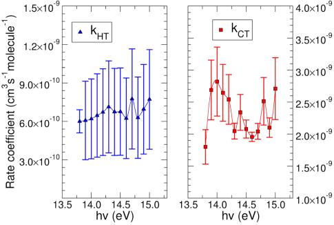
Fig. 4 Rate coefficient for the reaction of  $CO_2^+$  with water. On the left panel is reported the k for the HT channel as a function of the photon energy. On the right panel the rate coefficient for the CT process is shown. See main text for further details.
