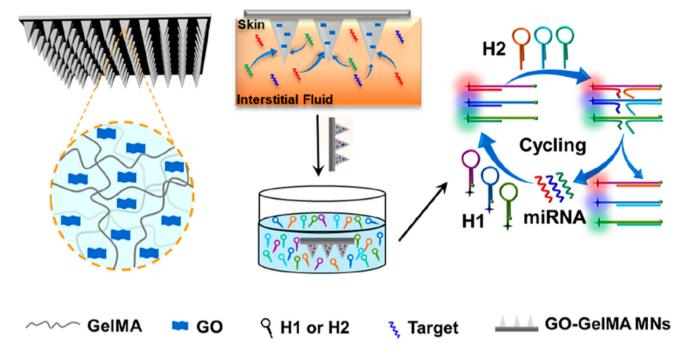
Fig. 7 Schematic illustration of GO-GelMA MNs used for interstitial fluid extraction and the detection of miRNA. Reprinted with permission from American Chemical Society,<sup>53</sup> Copyright 2023.
