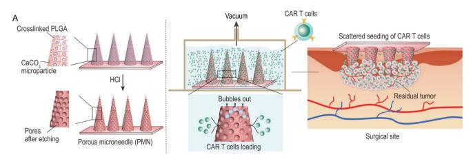
Fig. 9 Characterization of porous MN (PMN) patch for CAR T cell loading and delivery. (A) Schematic of PMN fabrication, CAR T cell loading, and implant of CAR-T-cell-loaded PMN (PMN@CAR T) within the tumor bed after surgery. Reprinted with permission from National science review, 64 Copyright 2021.
