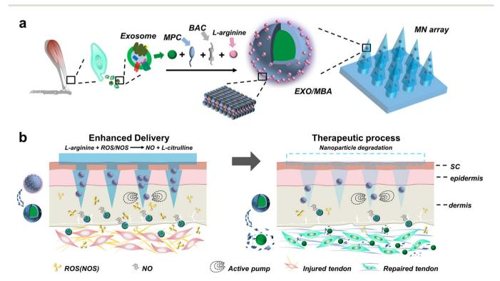
Fig. 12 Nitric oxide nanomotor driving exosomes-loaded microneedles schematic illustrations. (a) The manufacturing procedure of EXO/MBAloaded MN array. (b) The healing process of Achilles tendinopathy after application of EXO/MBA-loaded MN array. Reprinted with permission from American Chemical Society,73 Copyright 2021.
