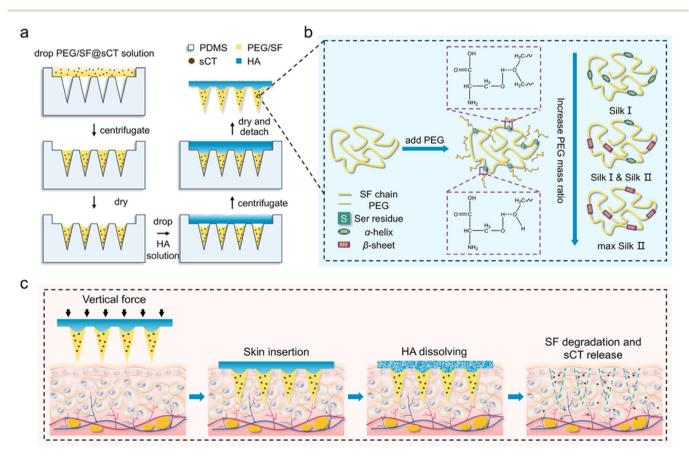
Fig. 5 Schematic illustrations of the fabrication process of HA-PEG/SF@sCT MNs (a), PEG-induced conformational transition of SF (b), and transmucosal delivery of sCT using the HA-PEG/SF@sCT MNs (c). Silk fibroin (SF); poly(ethylene glycol) (PEG); salmon calcitonin (sCT). Reprinted with permission from American Chemical Society,<sup>38</sup> Copyright 2023.
