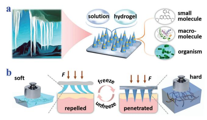
Fig. 8 Schematic illustrations of compositions and properties of ice MNs. (a) Ice–formation–inspired ice MNs can be made from soft materials such as solutions and hydrogels, and can carry diverse actives including small molecules, macromolecules, and living organisms. (b) Scheme of transformation from softness to hardness realized by freezing processes. Reprinted with permission from American Chemical Society Advanced Science published by Wiley-VCH GmbH, 61 Copyright 2021.
