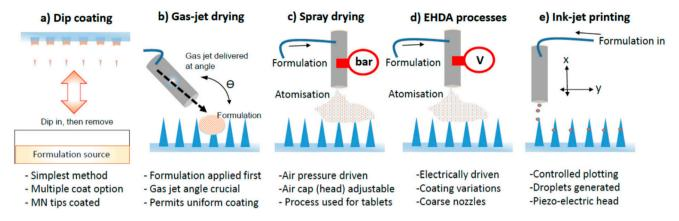
Fig. 3 Illustrated examples of techniques used to coat MNs. (a) Dip coating; (b) gas-jet drying; (c) spray drying; (d) EHDA processes; (e) ink-jet printing. Reprinted with permission from MDPI,<sup>20</sup> Copyright 2015.
