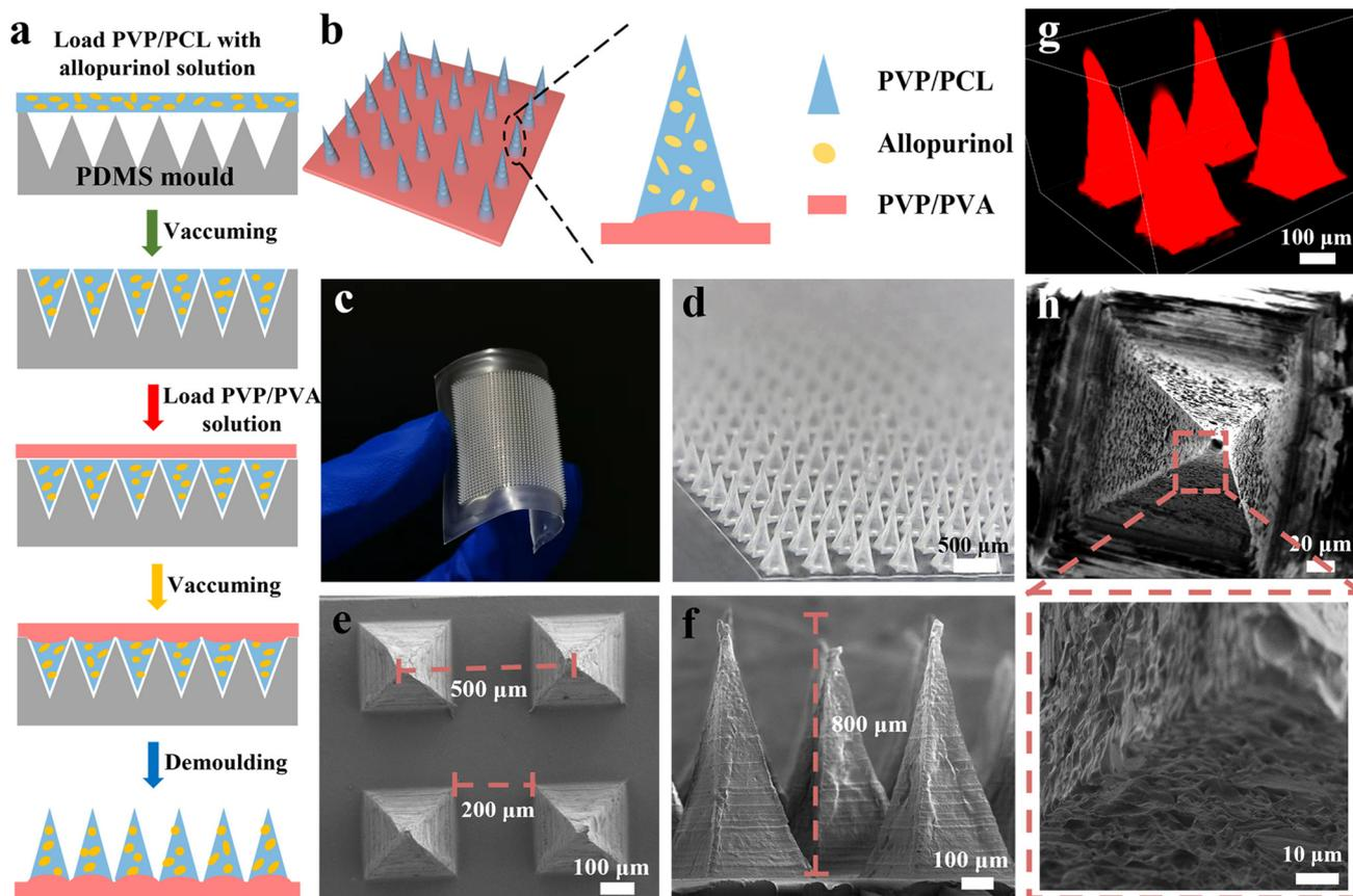
**Fig. 1** Schematic of the fabrication process of MNs (a), schematic structure of MNs (b), digital images of the as-fabricated MNs (c and d), SEM images of PVP/PCL MNs (e and f), the confocal image of MN arrays (g), and the porous structure of MNs formed by the rapid dissolution of PVP (h).
