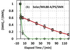
Fig. 9 Effect of drinking water and deionized water (control) on the degradation of SMX as a function of time (min): (a) in the UVA/MIL88-A/PS/SMX and (b) in the solar/MIL88-A/PS/SMX systems. Experiments were done in a rotisserie shaker. Experimental conditions: [SMX]0 = 5 mg L $^{-1}$ , [PS] = 2 mM, and [MIL88-A]0 = 125 mg L $^{-1}$ . Error bars are calculated as  $ts/\sqrt{n}$ , where absent bars fall within the symbols.
