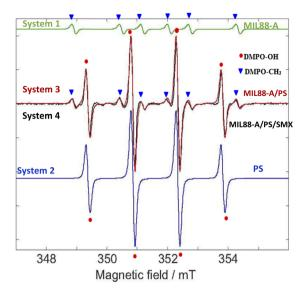
Fig. 11 EPR spectra. Green – simulated EPR spectrum for trapped methyl radicals. aN =1.58 mT and aH =2.28 mT. Blue – simulated EPR spectrum for trapped hydroxyl radicals. aN = 1.49 mT and aH = 1.49 mT. Red – the sum of the above two simulated trapped radical spectra. Black – experimental EPR spectrum under the following experimental conditions: [PS] = 2.5 mM, [MIL88-A] = 12.5 mg L $^{-1}$ , and [DMPO] = 100 mM.
