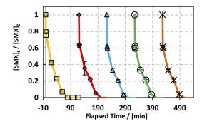
Fig. 4 Recyclability experiments of MIL88-A in the UVA/MIL88-A/PS/ SMX system. Experimental conditions:  $[SMX]_0 = 5 \text{ mg L}^{-1}$ ;  $[PS]_0 = 2$ mM; [MIL88-A] = 125 mg L<sup>-1</sup>; error bars are calculated as  $ts/\sqrt{n}$ , where absent bars fall within the symbols.
