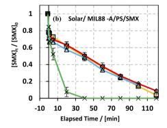
Fig. 8 Effect of bicarbonate concentration on the degradation of SMX as a function of time in different systems: (a) UVA/MIL88-A/PS/SMX and (b) solar/MIL88-A/PS/SMX systems. Experimental conditions:  $[HCO_3^-] = 1-100 \text{ mM}, [SMX]0 = 5 \text{ mg L}^{-1}, [PS]0 = 2 \text{ mM}, and [MIL88-1]$ A]0 = 125 mg L<sup>-1</sup>. Error bars are calculated as  $ts/\sqrt{n}$ , where absent bars fall within the symbols.
