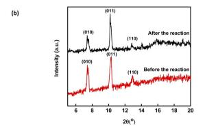
Fig. 5 (a) SEM images of recycled MIL88-A and (b) XRD pattern of new  $\emph{vs.}$  used MIL88-A crystals.
