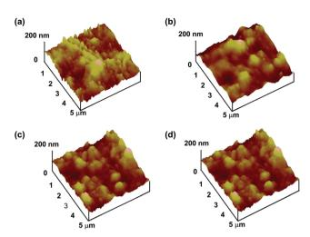
Fig. 6 High-resolution AFM images of (a) untreated PEEK, (b) r-PMB-PEEK, (c) di-PMB-PEEK, and (d) tri-PMB-PEEK surfaces.
