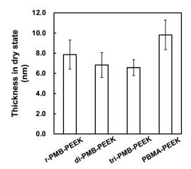
Fig. 4 Thicknesses of the PMB layers after photoreaction.
