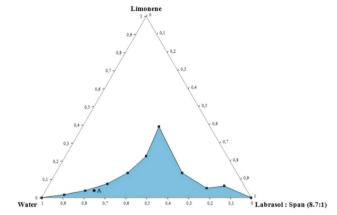
**Fig. 2** Pseudo-ternary phase diagram of the system consisting of limonene as the oil phase, Labrasol<sup>®</sup> and Span 80 as surfactants and distilled water as the continuous phase. Composition is in weight ratios. The monophasic region of the system is shaded with blue color and clear area is the multi-phase region. Point A corresponds to the following composition: 78.7% water, 17.5% surfactants and 3.8% limonene. Temperature was kept constant at 25 °C.
