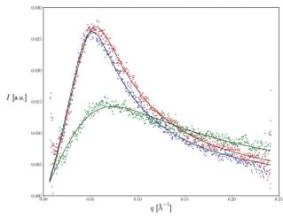
Fig. 5 SAXS spectra of the empty microemulsion (blue line) and that loaded with the conjugated polymers (red line - microemulsion with PBDT-DPP, green line - microemulsion with PIDT-TDQ). Lower panel: Processed data, subtracting the buffer contribution. Linear scale. Continuous black lines: best fits. Measuring temperature: 25 °C
