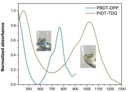
Fig. 6 UV-Vis spectra of the PBDT-DPP PIDT-TDQ O/W microemulsions
