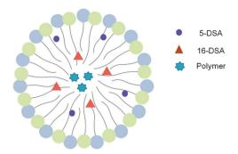
Fig. 4 Schematic representation of the localization of spin probes and polymer molecules in an oil droplet of the O/W microemulsion based on FPR results
