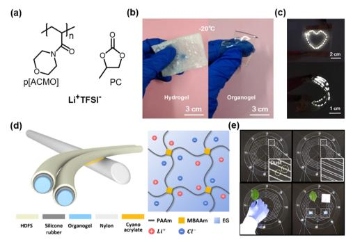
Fig. 6 Organogel-based SICs. (a) One example of organogel-based ionic conductors. (b) The organogel ionic conductor is mechanically conformable at -20 °C. (c) The organogel ionic conductor as a stretchable electrode. Reproduced with permission from ref. 61. Copyright 2019, The American Chemical Society. (d) Another example of an organogel-based ionic conductor and its components. (e) Demonstration of artificial spiderwebs. Reproduced with permission from ref. 35. Copyright 2020, AAAS.
