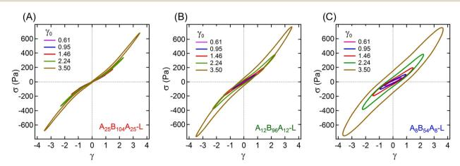
Fig. 3 Lissajous plots obtained from amplitude sweep experiments displaying the shear stress ( $\sigma$ ) vs. intracycle strain ( $\gamma$ ) for (A)  $A_{25}B_{104}A_{25}$ -L, (B)  $A_{12}B_{96}A_{12}$ -L, and (C)  $A_8B_{54}A_8$ -L for  $\gamma_0\approx0.61$ , 0.95, 1.46, 2.24, and 3.50. The experiments were performed using oscillatory frequency ( $\omega$ ) of 1 rad s<sup>-1</sup>.
