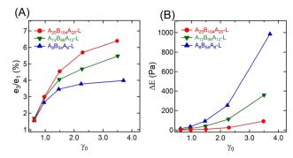
Fig. 5 (A) Ratio of Chebyshev elastic coefficients  $(e_3/e_1)$ , and (B) energy dissipated ( $\Delta E$ ) over a strain cycle for  $A_{25}B_{104}A_{25}-L$ ,  $A_{12}B_{96}A_{12}-L$ , and  $A_8B_{54}A_8$ -L as a function of  $\gamma_0 = 0.61-3.50$
