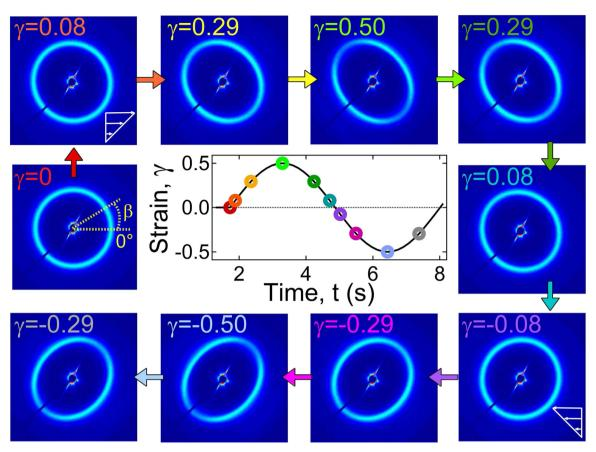
Fig. 10 Change of microstructure in a strain cycle for the  $A_{12}B_{96}A_{12}$ -H at room temperature. The strain ( $\gamma$ ) cycle as a function of time at the center also indicates the  $\gamma$ -values at which 2D scattering patterns were obtained from RheoSAXS experiments (in a clockwise direction).
