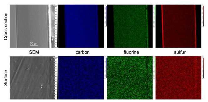
Fig. 4 SEM and EPMA element mapping images (blue: carbon, green: fluorine, and red: sulfur) of cross section and surface of the ionic SMP gel sensor with PEDOT: PSS electrodes on both surfaces of the gel ( $W_{IL}$  = 25 wt%).
