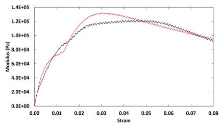
Fig. 7 Stress-strain curves for 2-18 at room temperature: trial 1 (black) and trial 2 (red).
