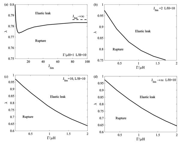
Fig. 8 Leak by elastic deformation and leak by rupture are demarcated on planes of various axes. (a) The diagram in the  $J_{lim}$ - $\lambda$  plane for strain-stiffening seals with the fixed  $\Gamma/\mu H$  and L/H. (b) The diagrams in the  $\Gamma/\mu H - \lambda$  plane for strain-stiffening seals with the fixed  $J_{\text{lim}}$  and L/H. (c) The diagrams in the  $\Gamma/\mu H - \lambda$  $\mu H - \lambda$  plane for neo-Hookean seals with the fixed L/H.
