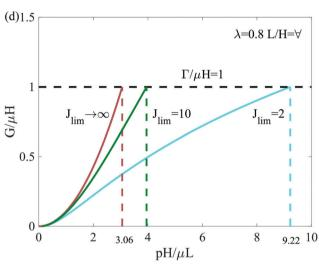
Fig. 6 A model of rupture. (a-c) The model assumes a debonded region of length  $l_c$  located at the bottom of the upstream front of the seal. (d) The relation between energy release rate G and pressure p. A strain-stiffening material will enhance the critical pressure of rupture compared to a neo-Hookean material
