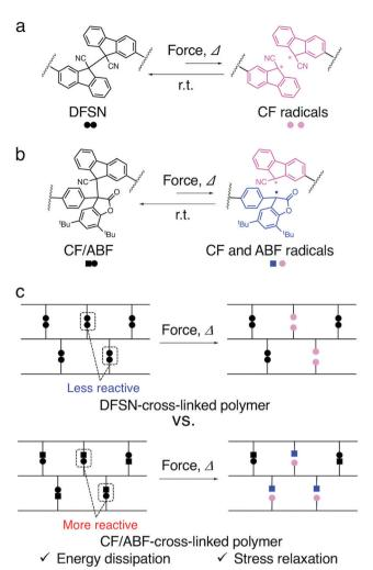
Fig. 1 (a) Equilibrium between DFSN and its radical species. (b) Equilibrium between CF/ABF and its radical species. Illustration of (c) a DFSNcross-linked polymer and a CF/ABF-cross-linked polymer, as well as the mechanism of energy dissipation and stress relaxation
