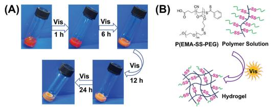
Fig. 1 (A) Images of hydrogel formation under visible light irradiation. (B) The schematic for formation of the crosslinked network.
