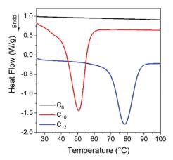
Fig. 2 After 1 day of isothermal crystallization at room temperature, C<sub>10</sub> and  $C_{12}$  show clear melting peaks whereas  $C_8$  still exhibits no melting transition.
