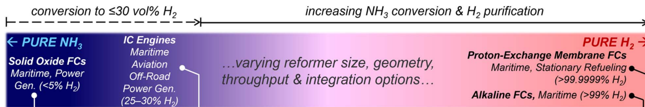
Scheme 1 Spectrum of \text{NH}_3 -capable internal combustion (IC) and fuel cell (FC) technologies for air, sea and land mobility and for stationary applications as a function of \text{NH}_3 conversion ( i.e. , \text{H}_2 fraction in reformat). Note that additional hydrogen purification is required following catalytic \text{NH}_3 reforming for FC applications.
