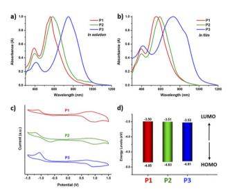
Fig. 5 Characterization of polymers P1, P2 and P3 (a) UV-vis absorption spectra in chloroform solution; (b) as a thin film. (c) cyclic voltammograms as a thin film (scan rate 100 mV s $^{-1}$ ) and (d) HOMO–LUMO energy level diagram obtained using CV measurement.
