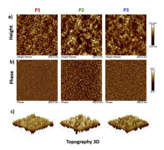
Fig. 9 Tapping-mode AFM images of (a) the height, (b) phase with a 0.4  $\mu$ m  $\times$  0.4  $\mu$ m scan size and (c) 3D-topography of copolymers P1–P3
