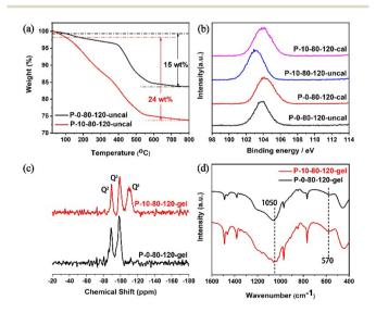
Fig. 3 (a) TG curves of P-10-80-120 and P-0-80-120 before calcination, (b) XPS spectra of Si 2p of P-10-80-120 and P-0-80-120 before and after calcination, (c) <sup>29</sup>Si MAS NMR spectra and (d) FT-IR spectra of the P-0-80-120 gel and P-10-80-120 gel.
