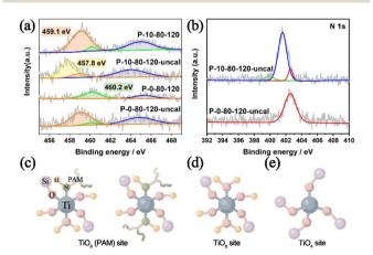
Fig. 5 (a) XPS spectra of Ti 2p in P-10-80-120 and P-0-80-120 before and after calcination, (b) XPS spectra of N 1s of P-10-80-120 and P-0-80-120 before calcination and proposed titanium active sites: (c) TiO<sub>6</sub> (PAM) site, (d) TiO<sub>6</sub> site and (e) TiO<sub>4</sub> site.
