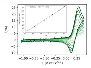
Fig. 1 Scan rate dependence of a 1 mM solution of 1 in in 2:1 THF/DFB + 0.2 M NaPF6 (from light to dark green: 0.05, 0.1, 0.2, 0.3, 0.4 and 0.5 V s $^{-1}$ , 3 mm GC electrode). Inset: evolution of the peak current as a function of the square root of the scan rate.
