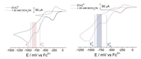
Fig. 1 CV of  $[Cu^{II}L(NCCH_3)]^{2+}$  (2 mM) before and after the addition of 10 equivalents (20 mM) ClCH<sub>2</sub>CN (left, **1a**) and BrCH<sub>2</sub>CN (right, **1b**) (at a scan rate of 100 mV s<sup>-1</sup>: highlighted shaded areas show the potential window for forming  $[Cu^{II}L(CH_2CN)]^+$ .
