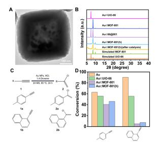
Fig. 5 (A) TEM images of Au $\subset$ MOF-801(h). (B) PXRD patterns of Au $\subset$ UiO-66, Au $\subset$ MOF-801, and Au $\subset$ MOF-801 before and after catalysis. (C) Au catalyzed reaction of terminal alkynes with HCl. (D) The conversion of 4-ethynyltoluene and 1-ethynylnaphthalene over different catalysts after 24 h of the reaction with HCl.
